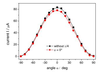
Fig. 3: Current I as a function of the analyzer position  $\alpha$ : without quarter wave plate (black) and with quarter wave plate at position  $\phi = 0^{\circ}$  (red). The solid lines are guides to the eyes only.
