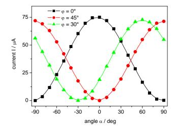
Fig. 5: Current I as a function of the analyzer position  $\alpha$  for various half wave plate positions  $\phi.$  The solid lines are guides to the eyes only.
